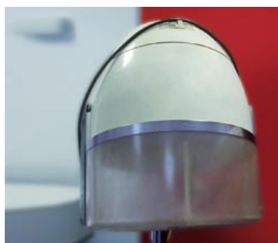
Figure 47 Asbestos-containing commercial hairdryer
