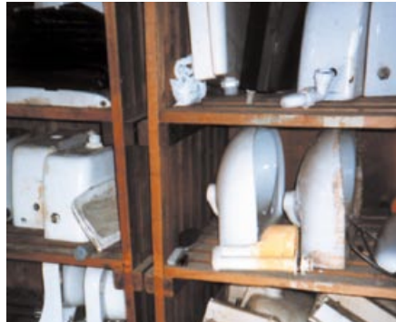
Figure 40 Asbestos-reinforced toilet cistern
