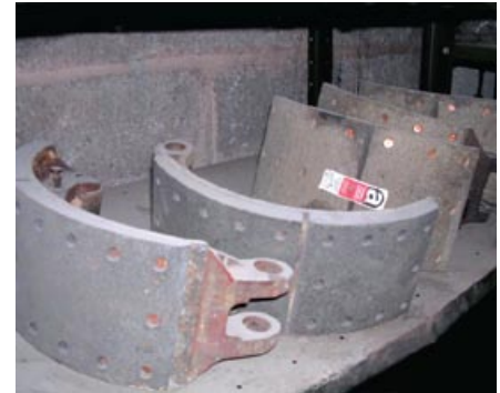
Figure 41 Asbestos brake linings for quarry vehicles
